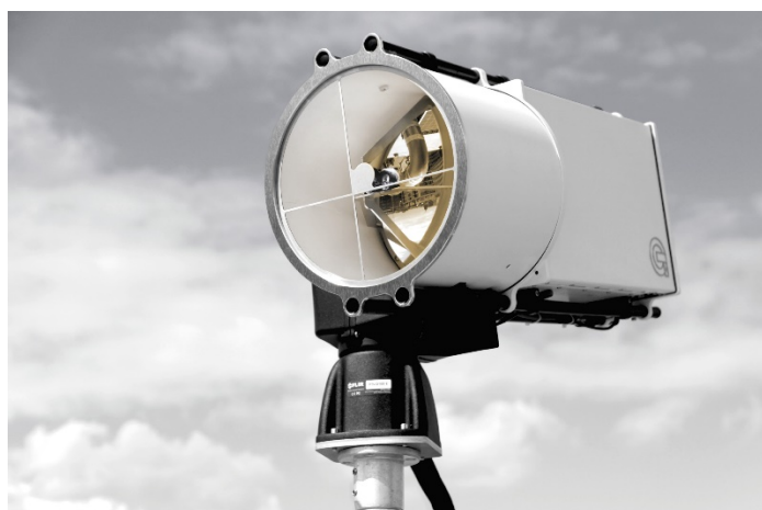
Figure 3: The scanfeld™ sensor unit is a scanning imaging FTIR spectrometer. The picture shows the sensor (white) with the large aperture infrared telescope head. The sensor is moved continuously by a pan-tilt unit (black) to scan the area of interest.
