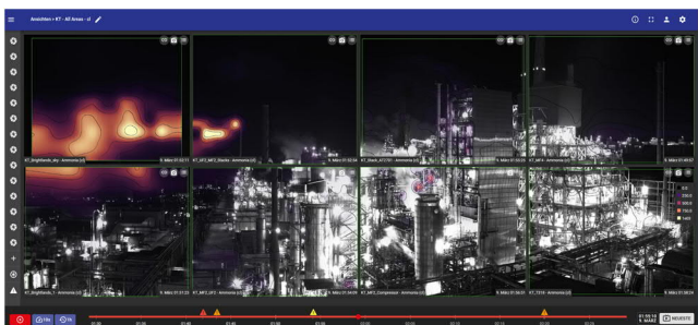
Figure 3: Data example of eight scan areas of a production site. The scan areas are sequentially scanned and displayed in a multi-view user interface.
