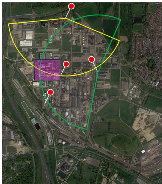
Figure 13: A sketch for an installation of two additional sensor units to monitor the entire Chemelot north chemical site. The monitoring area covers 1.6 km 2 . The monitoring solution covers 8 toxic or flammable gases.
