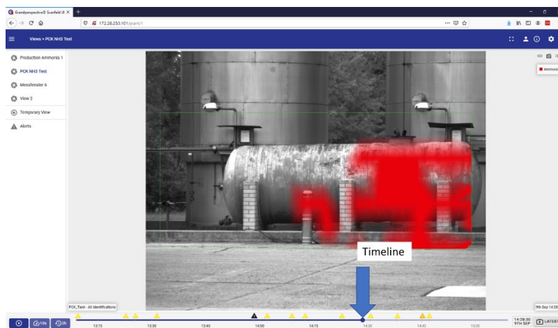
Figure 6: Screenshot of the user interface that shows how the point-of-view visualization of a gas cloud is organized together with the incident alert in a time line.
