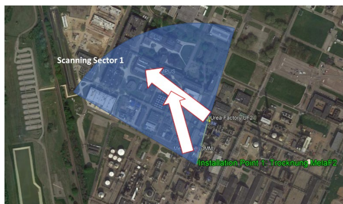
Figure 9: The image shows the installation point and the viewing area that effectively oversees the entire campus. The white arrows indicate the potential propagation direction of a release from one of the four stacks. The location of the sensor unit enables the continuous monitoring of a gas cloud from the point of release on over the entire monitoring area.
