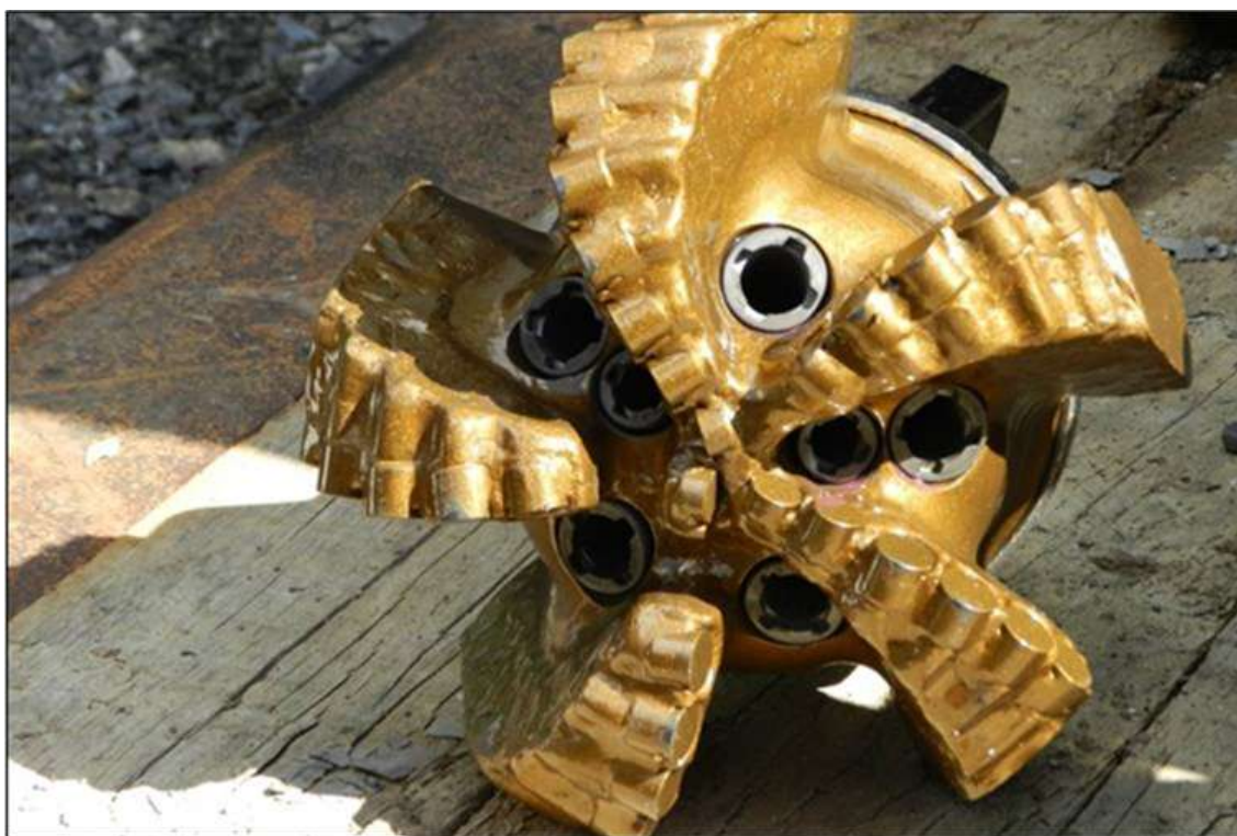
Figure 9.1: Photo of a drill bit with a Polycrystalline Diamond Compact (PDC) cutter
