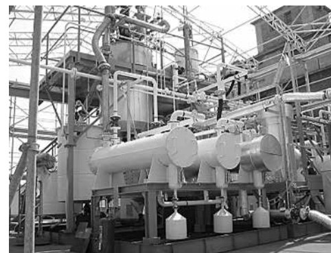
Figure 15: The Indirect Thermal Desorption Unit (ITDU) at Spolana Neratovice, Czech Republic.
