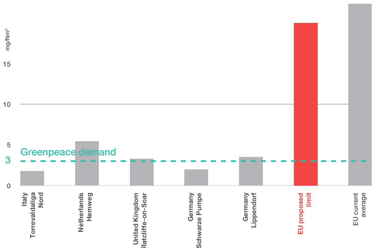
Figure 3: Examples of EU power plants with PM emissions far below proposed standard.
